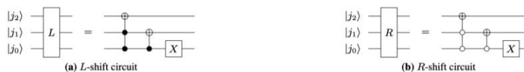
Figure 3. Shift operators (quantum “transition matrices”) and their corresponding circuits. Schematic taken from https://arxiv.org/abs/2203.10236 .
